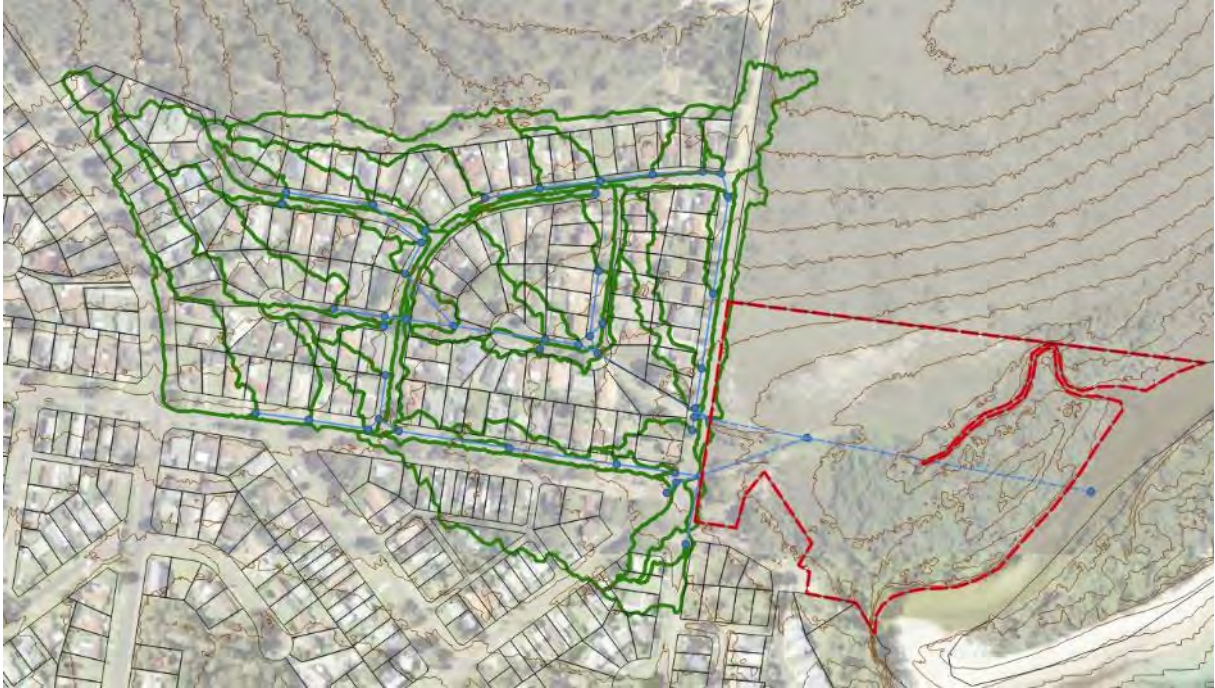
Figure 4: Catchment Plan – Existing Residential Catchment (Catchments in Green, Pipes as Solid Blue Lines, Drainage Nodes as Blue Dots, Open Channels and Blue Dashed Lines)
